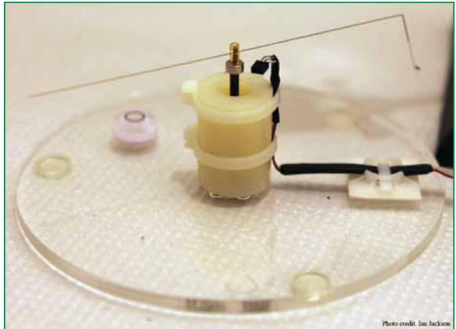
**Figure 1.** A laboratory flight mill used to investigate movement of insects, including Asian citrus psyllid.
