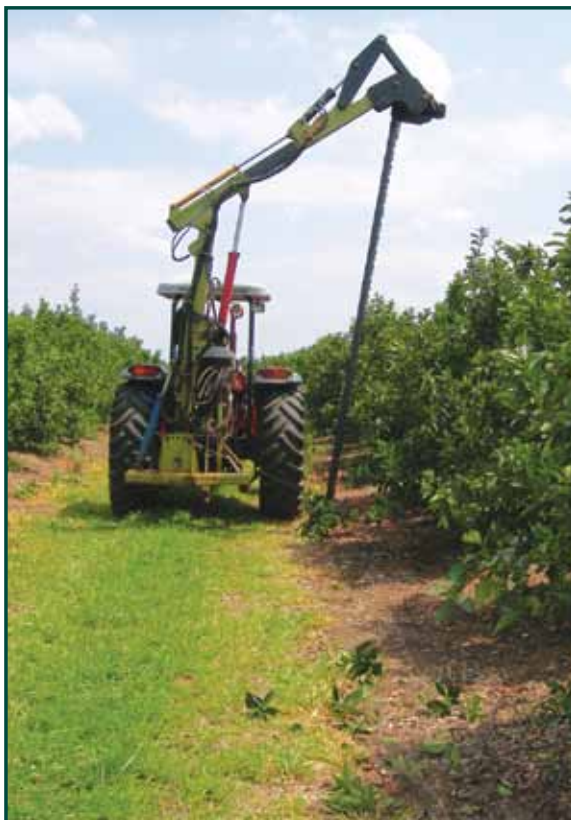
Figure 3. Tractor-mounted, sickle-bar hedging machine used for light trimming of citrus canopies in Brazil
