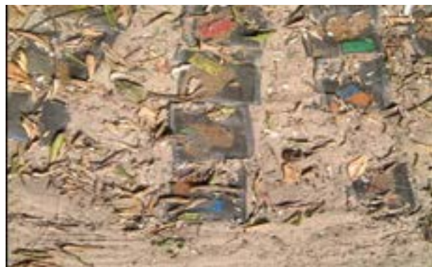
Figure 9. Current research showing porous bags containing CRF nutrient sources. Materials within the bag are exposed to both rainfall and irrigation. Contents of the bags are analyzed at selected time intervals to indicate the nutrient release rates of the CRF sources.
