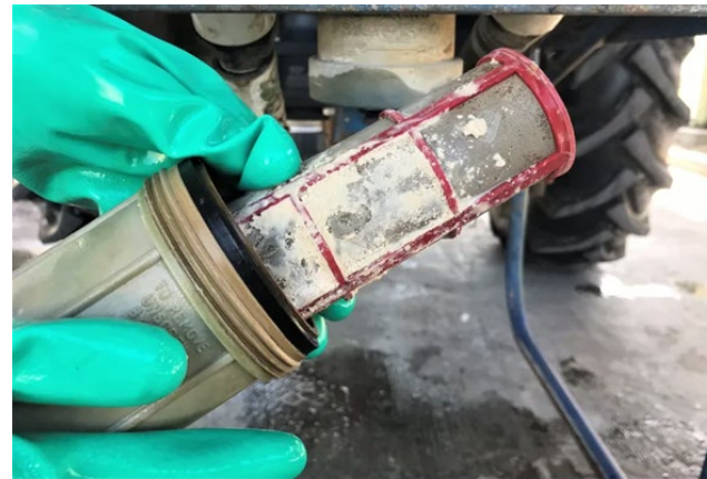
clogged sprayer filter
