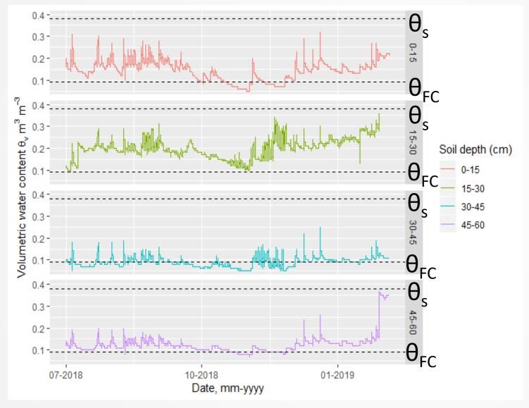
Soil moisture remained above field capacity at 0-6-inch, 6-24-inch depth most of the time and close to field capacity at 12-18-inch depth
