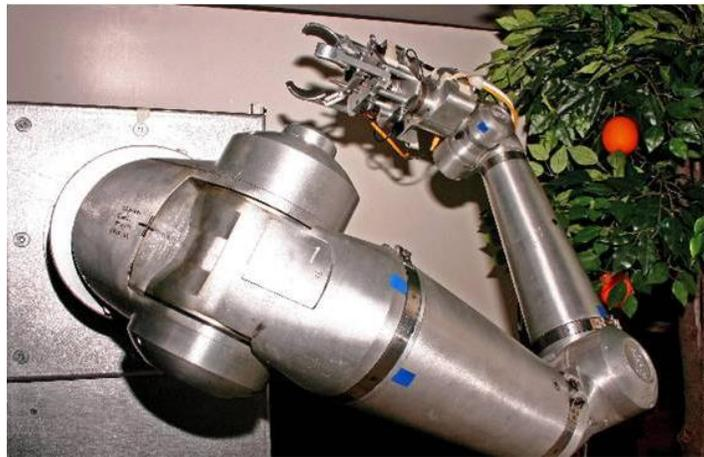
First end effector with force/torque sensor used in harvesting motion testing.
