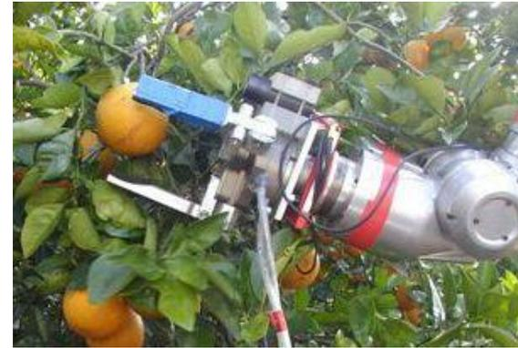
3rd and 4<sup>th</sup> prototype using pneumatic actuation and vacuum grip.
