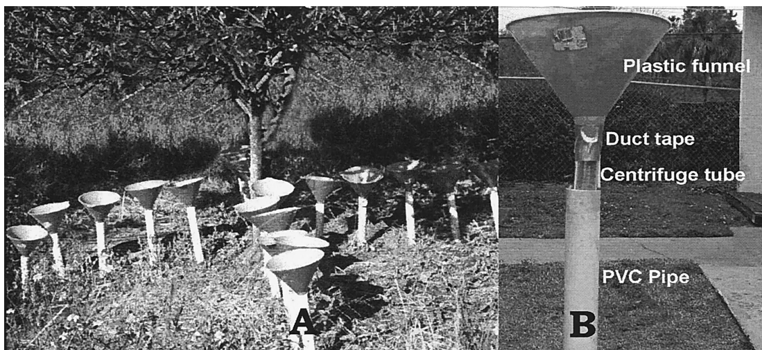
Fig. 1. (A) Traps installed under a citrus tree. (B) Trap detail.
