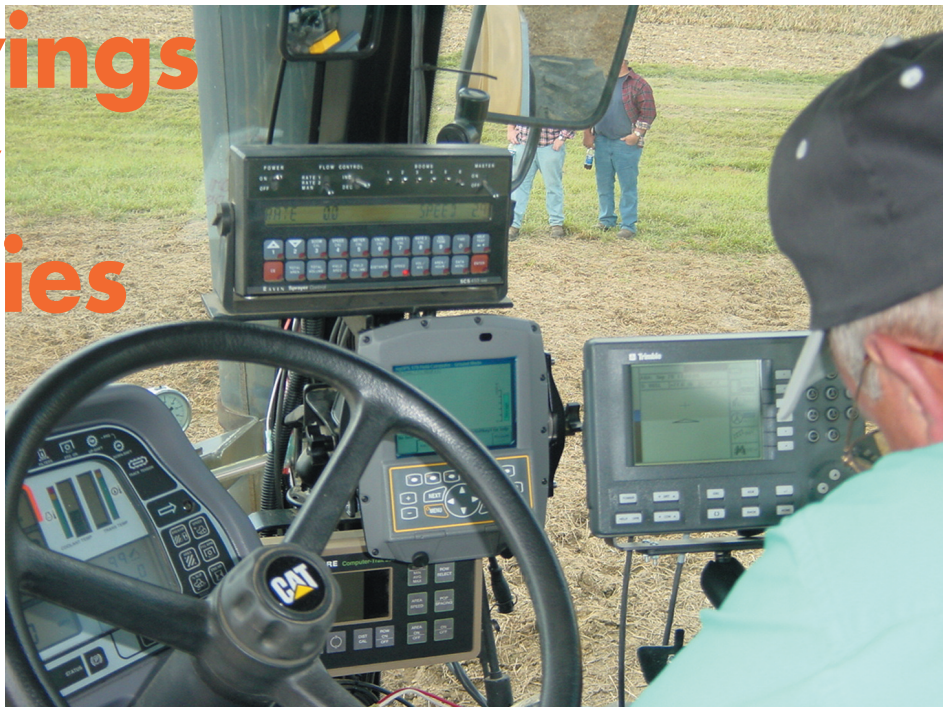
A tractor equipped with a variable rate controller, guidance system and other equipment can potentially increase the productivity of the operator.
