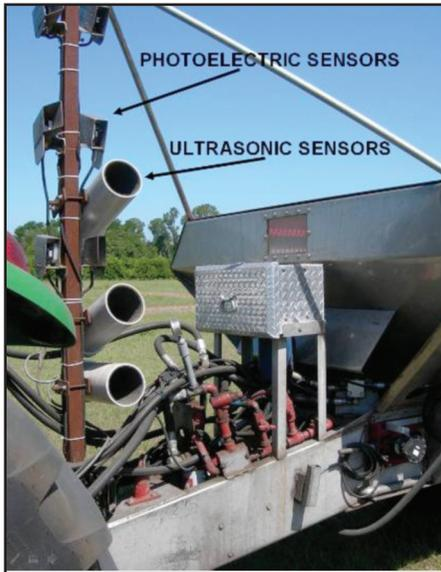
Figure 1. Left to right: Canopy sensors, sensor control box, VRF computer controller.
