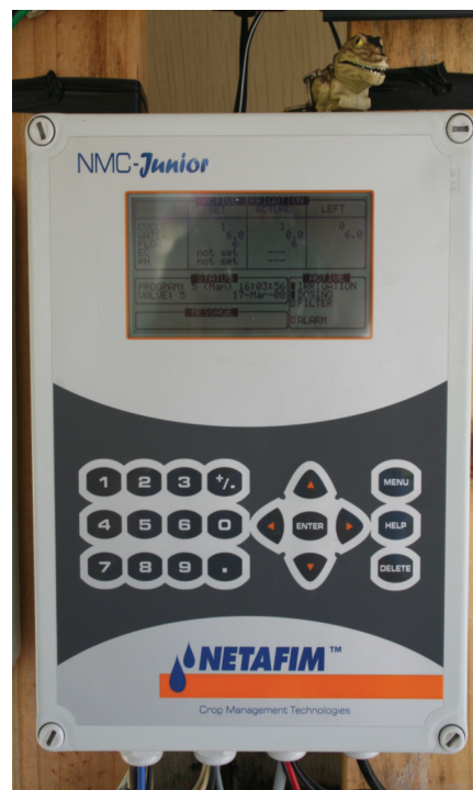
Figure 1. An example of a controller suitable for automated, remote-controlled citrus irrigation
