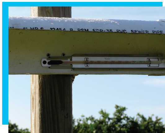
Collection of accurate site specific minimum temperature data begins with a properly shielded grove thermometer. This allows growers to fine-tune minimum temperature forecasts.
