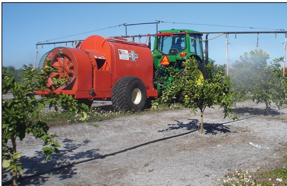
Figure 2. Young solid-set trees being sprayed with an automatic VRT hoop spray boom.
