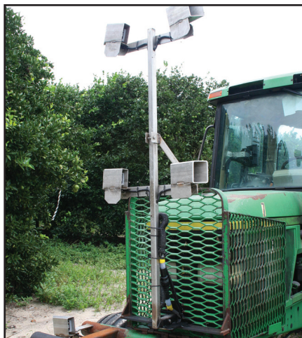
Figure 3. Enhanced VRT system, from left: optical canopy sensors mounted to the front of a tractor, VRT control box in the tractor cab, and the handheld setup computer
