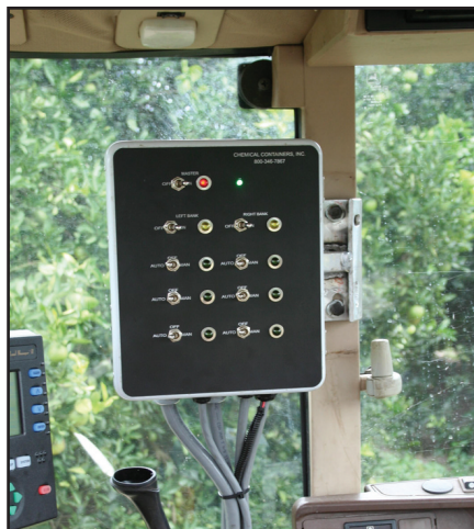
Figure 3. Enhanced VRT system, from left: optical canopy sensors mounted to the front of a tractor, VRT control box in the tractor cab, and the handheld setup computer
