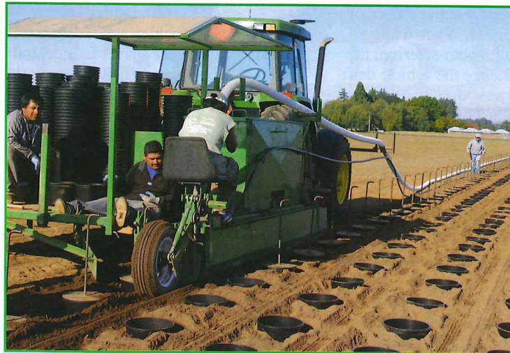
An auto-steer tractor used for planting containerized trees in an open field nursery.
