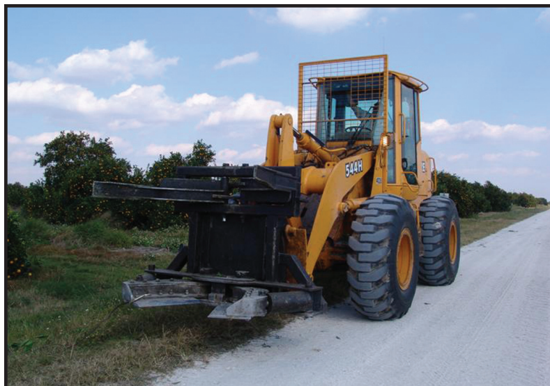
Figure 1 (left). Front-end loader used in clipping citrus trees with tree shear attachment.
