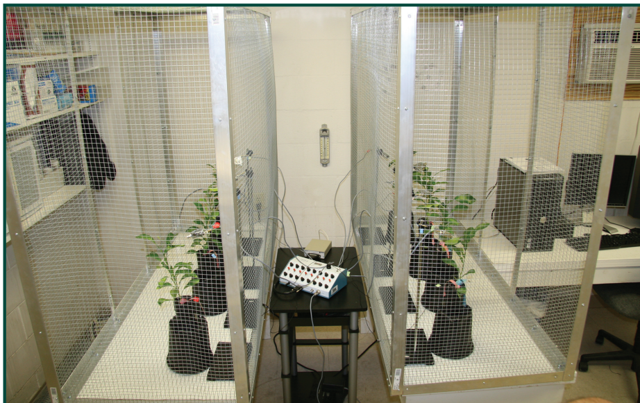
Figure 1. Electrical penetration graph (EPG) monitor for recording psyllid feeding behaviors on insecticide-treated and untreated citrus.
