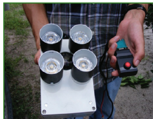
Figure 1. Optical sensors used for disease detection: (top) four-band active sensor; and (left) five-band passive sensor.
