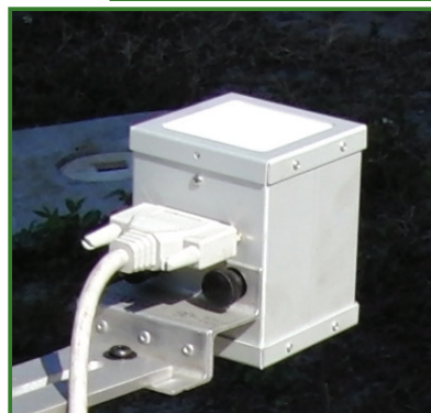
Figure 1. Optical sensors used for disease detection: (top) four-band active sensor; and (left) five-band passive sensor.
