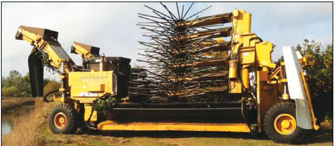
Figure 1. A self-propelled canopy shaker equipped with a catch frame is currently being used to harvest Florida's sweet orange crop.
