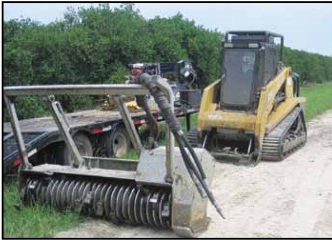
Fig. 1. Cost of removal of HLB trees with tree grinder is $4.50 to $5.50 per tree. Chipped material remains in the grove middles.
