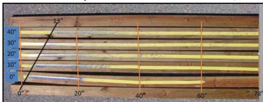
Figure 8. The distance of the deposited spray for the OC nozzle angles of 0°, 10°, 20°, 30° and 40° as shown on the bottom to top target strips, respectively. The black line, beginning at the bottom lefthand side of the photo, shows the increasing distance from the nozzle where the spray begins to reach the target with increasing nozzle angle. At 0°, the target is contacted near the nozzle tip, and at 40°, it approaches 13 inches from the nozzle.
