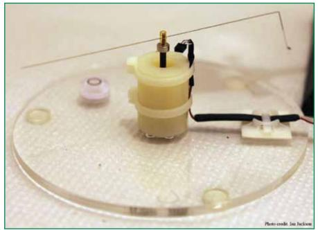
Figure 1. A laboratory flight mill used to investigate movement of insects, including Asian citrus psyllid.
