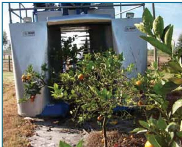
Figure 2 (below). A BEI over-the-row blueberry harvester is being tested for harvesting young citrus trees.
