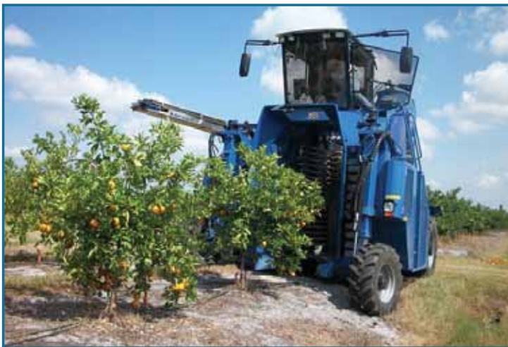
Figure 1 (right). An Oxbo over-the-row olive harvester is being tested for harvesting young citrus trees.
