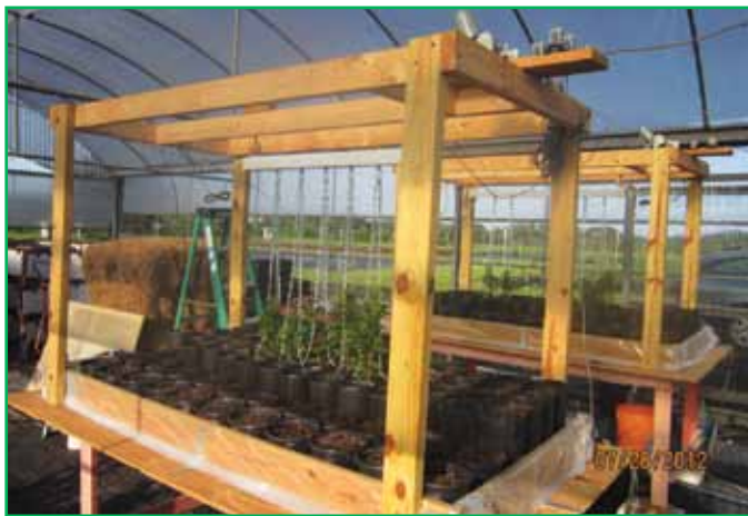
Figure 2. Ebb-and-flow tables during the testing stage. Plants in the middle were used to test and refine the automated weighing of five plants in the middle of a table to determine daily tree water use.
