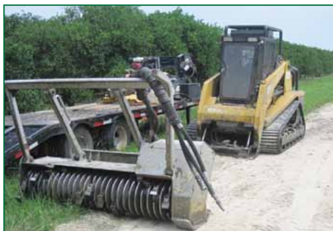
Removal of HLB infected trees has been a hard sell for growers. In 2011, cost of removal by a tree grinder was $4.50 to $5.50 per tree.
