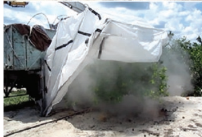
BELOW: Figure 4: A system for in-field thermotherapy using steam as the heat source mounted on a 5-ton surplus military truck (M1078).
