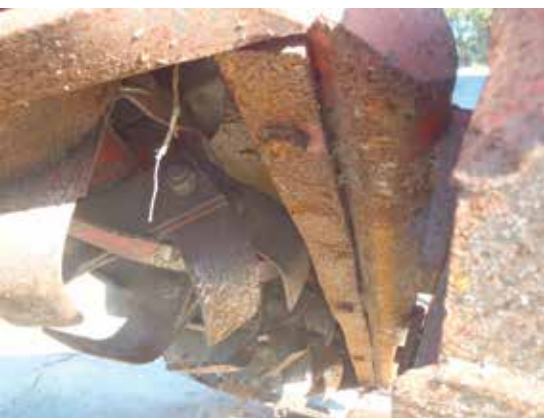
Figure 5. Side operating tree hoe: side view (top photo) and cultivator tines seen from below (bottom photo). Photo credit: Phil Stansly
