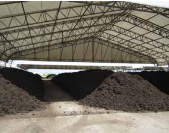
Figure 1. Overview of windrow composting of yard-trimming waste and biosolids at the Lee County Composting Facility in Felida. Photo credit: Monica Ozores-Hampton
