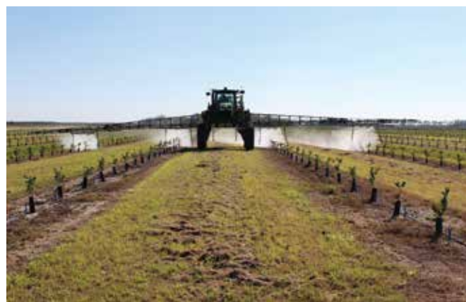
Figure 1. This crop sprayer has been modified to spray up to five rows of citrus trees in a single pass.
