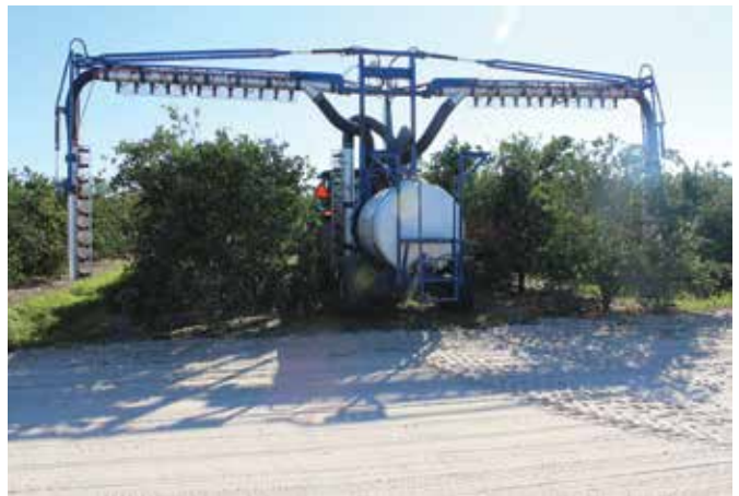
Figure 3. An over-the-row citrus sprayer can cover two rows in a single pass.
