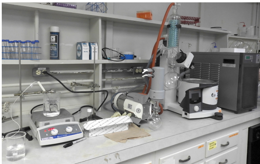
High-tech equipment at the Citrus Research and Education Center used in flavor research includes a liquid chromatography/mass spectrometer (top) as well as a rotary evaporator with chiller and vacuum pump (bottom).
