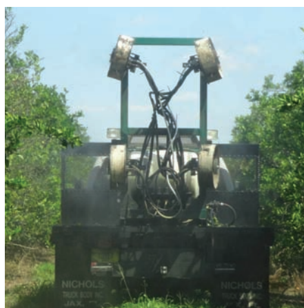
Figure 2. Proptec rotary atomizer sprayer for low-volume application
