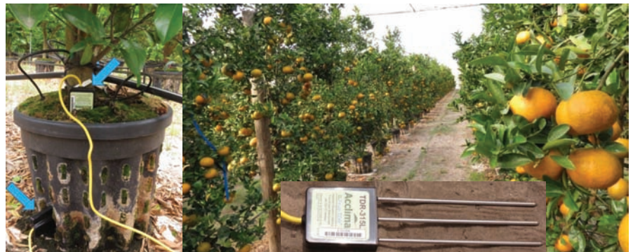
Figure 1. Acclima time-domain reflectometry (TDR) soil-water sensors are installed in pots used in hydroponically grown citrus under protective screen. The upper arrow shows the vertically installed sensor, and the lower arrow shows the horizontally installed sensor. The inset figure shows details of the three-pronged TDR sensor.
