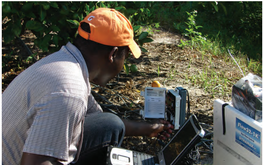
Data can be downloaded from soil moisture sensors to help growers make better irrigation decisions.
