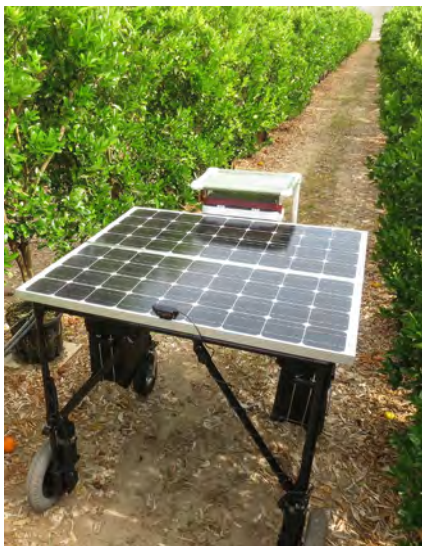
Figure 2. First prototype of a solar-powered robotic scout developed for citrus under protective screen groves
