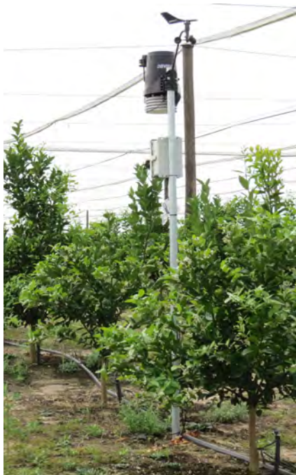
Figure 1. A grower's commercial citrus under protective screen grove includes a wireless weather station with TDT soil sensors in 1-year-old trees.
