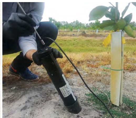
Figure 2. Minirhizotrons (left) and a camera system (right) are used for in-field imaging of young citrus tree roots.
