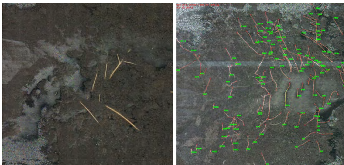
Figure 3. A minirhizotron imaging system captured images of fibrous roots from young citrus trees grown in a Southwest Florida grove. The photo on the right shows the tracing to calculate root length and other root parameters.
