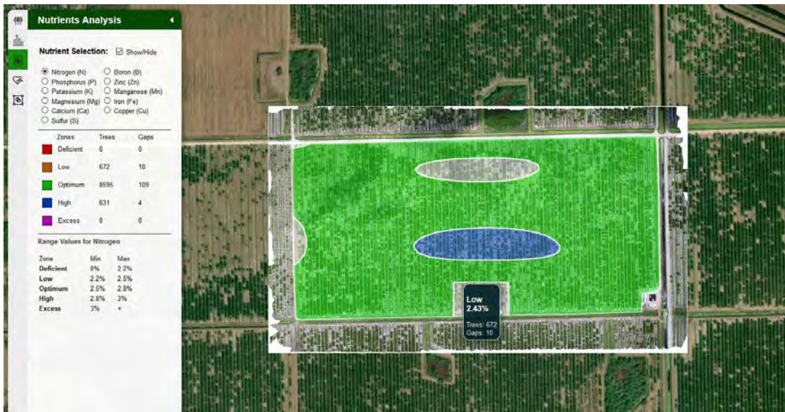
Figure 2. This fertility map was developed in Agrovion from data collected from an unmanned aerial vehicle equipped with a multi-spectral camera. Nutrient levels for zone development are based on University of Florida Institute of Food and Agricultural Sciences recommendations.
