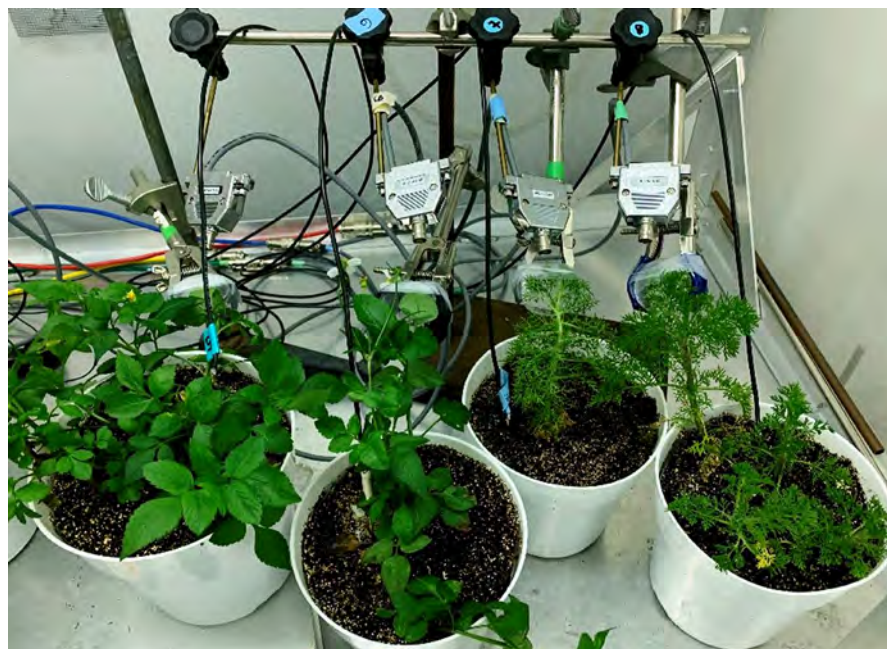
Figure 3. An experiment was set up to record psyllid feeding on weeds using electrical penetration graph technology.
