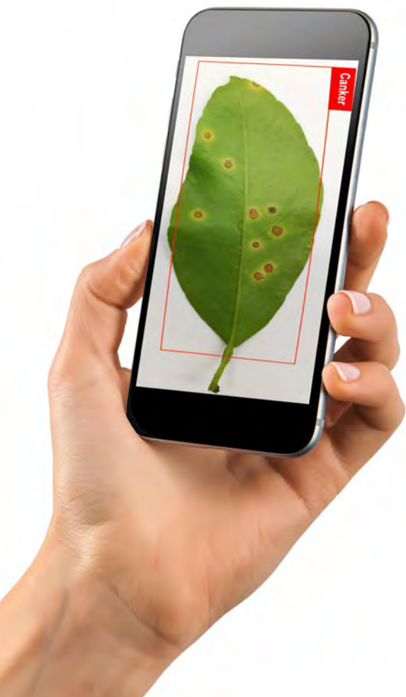
Figure 1. Automatic identification of leaf symptoms by machine vision uses deep-learning artificial neural networks.
