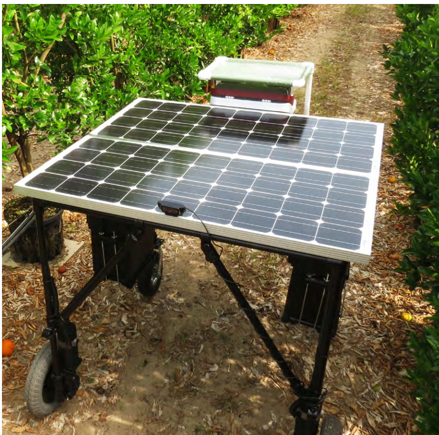
Arnold Schumann's psyllid scouting vehicle seeks to attract, capture and identify flying insects in a "smart" trap.
