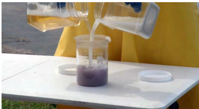
Figure 3. Chemical incompatibility is shown in this jar test.
