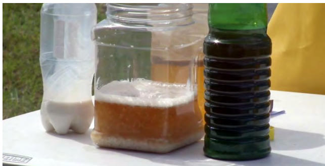
Figure 2. This jar test demonstrates physical incompatibility.
