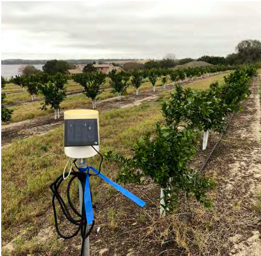
A soil sensor with a solar panel and rain gauge is installed in a row with 12 tons per acre of compost applied.
