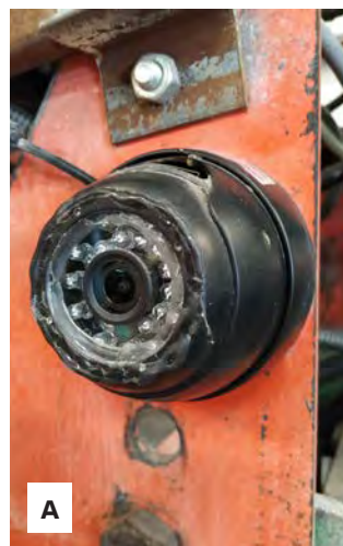
Figure 2. SmartSense for variable-rate sprayers: A) RGB camera installed on the sprayer and B) top view of the schematic of the positioning of cameras and lidar on the sprayer.
