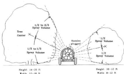
**Figure 1. Recommended nozzle arrangement and spray volume distribution.**
