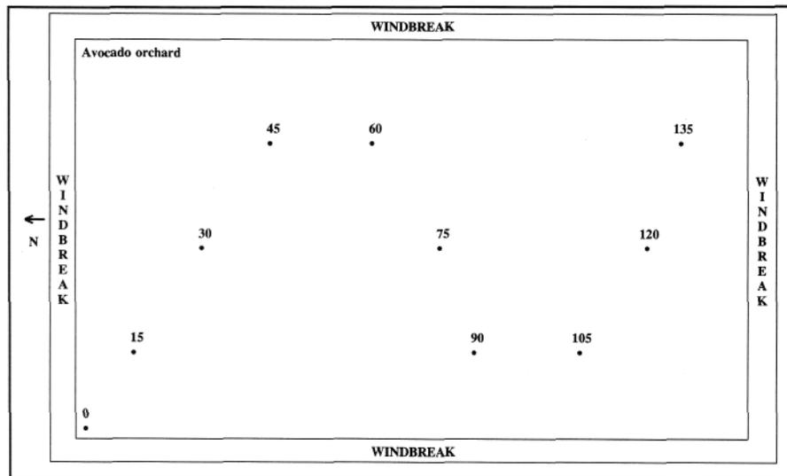
FIG. 1 Positioning of wind recorders in the avocado orchard. All positions are relative to the reference point 0.
