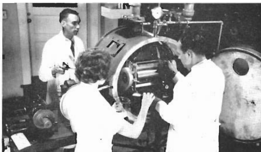
High Vacuum Double-Drum Dryer for Producing Powdered Citrus Juices— Florida Citrus Commission Research Fellows, E. L. Moore, E. Wiederhold, C. D. Atkins
