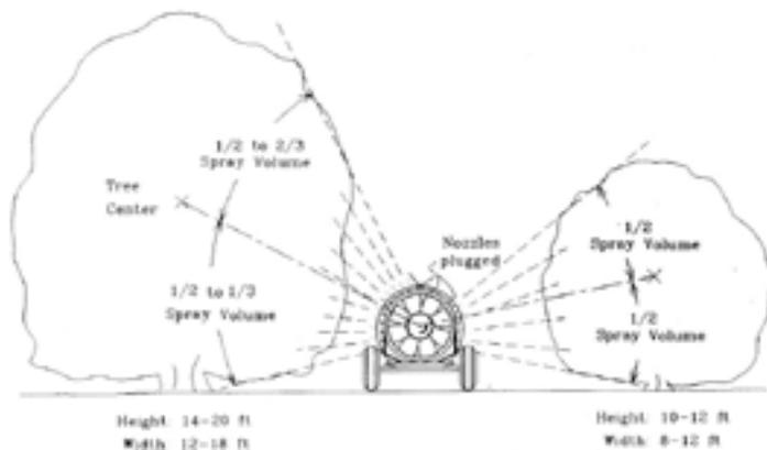
Figure 1. Recommended nozzle arrangement and spray volume distribution.
